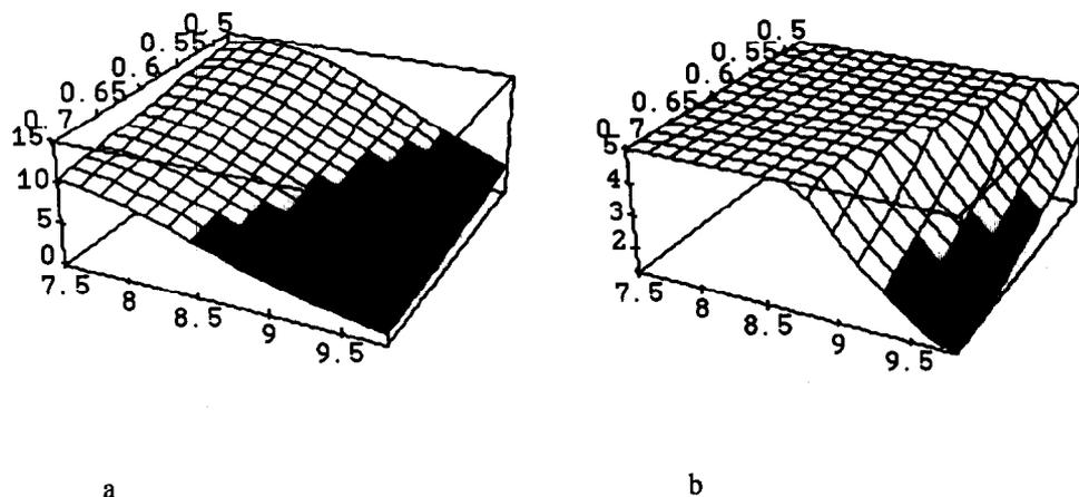
Fig. 2. (a) The resolution factor of the peak pair  $\text{HPO}_4^{2-}$ - $\text{NO}_3^-$  as a function of HBA concentration and pH of the mobile phase with constant methanol content (3%). Separation column: anion-exchange Hamilton PRP-X100. Regression and plotting model: logarithmic form of eqn. 2. (b) Three-dimensional plot of resolution factor surface,  $R_s$  ( $\text{HPO}_4^{2-}$ - $\text{NO}_3^-$ ) with  $R_s$  ranging from 1.2 to 5.0. Other conditions are the same as in (a).
