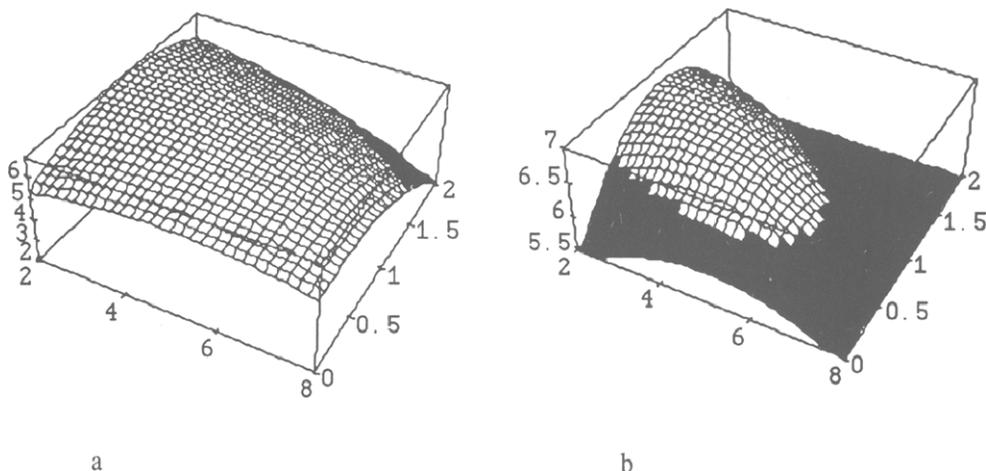
Fig. 5. (a) The peak height of  $\text{Cl}^-$  as a function of TBAI and KHP concentrations in the mobile phase with constant pH (5). Separation column: Whatman Partisil 10 ODS-3 RP. Regression and plotting model: normal form of eqn. 2. (b) Three-dimensional plot of peak height surface  $h(\text{Cl}^-)$  with  $h$  range from 5.5 to 7.0 (cm). Other conditions are the same as in (a).
