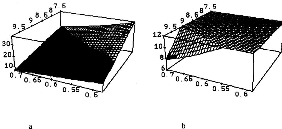
Fig. 3. (a) The retention time of the last peak,  $\text{SO}_4^{2-}$  as a function of HBA concentration and pH of the mobile phase with constant methanol content (3%). Separation column: anion-exchange Hamilton PRP-X100. Regression and plotting model: logarithmic form of eqn. 2. (b) Three-dimensional plot of retention time ( $t_R$ ) of  $\text{SO}_4^{2-}$  with  $t_R$  ranging from 6 to 12 (min). Other conditions are the same as in (a).
