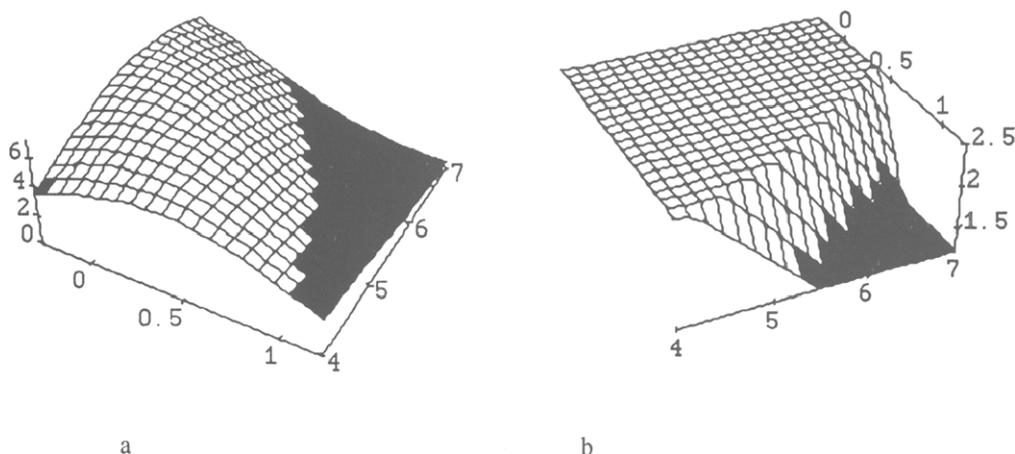
Fig. 4. (a) The resolution surface of the peak pair  $R_s(\text{NO}_3^-/\text{SO}_4^{2-})$  as a function of TBAI concentration and pH of the mobile phase with constant KHP concentration (1 mM). Separation column: Whatman Partisil 10 ODS-3 RP. Regression and plotting model: logarithmic form of eqn. 2. (b) Three-dimensional plot of resolution surface  $R_s(\text{NO}_3^-/\text{SO}_4^{2-})$  with  $R_s$  ranging from 1.2 to 2.5. Other conditions are the same as in (a).
